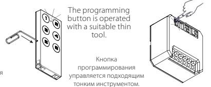
The programming button is operated with a suitable thin tool.
