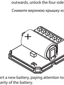
Insert a new battery, paying attention to the polarity of the battery.
